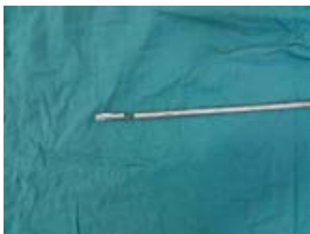
Fig. 1. Uncoiling flexible reamer in the distal part.
