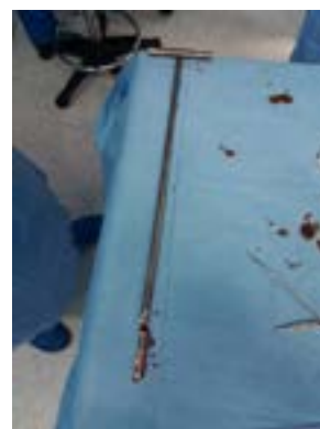
Fig. 4. Breakage in the shape part of the reamer.
