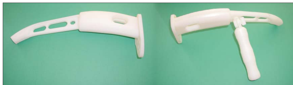
Fig. 13. Physical prototype of the Rasp Impactor made in the Rapid Prototyping technology
