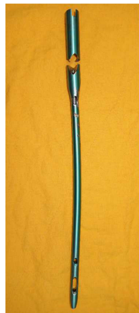
Fig. 5B. Retrieved long PFNA is broken at blade hole with rough fracture surface
